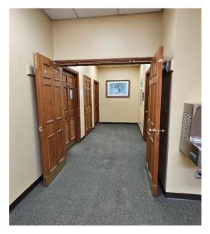
Second floor hallway leading to two public restrooms on the left side of the photo. The fire doors will be moved forward to align with the drinking fountain. This allows for the restroom doors to be relocated and the doorways to be expanded to meet ADA requirements. This area upstairs technically does not qualify for review as it was part of a 1985 addition.
